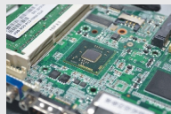
Onboard N2600 processor, power consumption 3.5W
