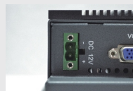
Phoenix terminal using fastening type power connector
