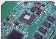
CPU and memory uses BGA surface mount technology, id temperature, pressure and long life solid capacitors implement
