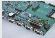
8 V ESD protection, TVS 600 surge protection, 2500VDC isolation serial magnetic coupling
