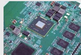
CPU and memory uses BGA surface mount technology, wide temperature, pressure and long life solid capacitors diskless installation of cable connections
