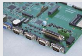
8KV ESD protection, TVS 600W surge protection, 2500VDC isolation serial magnetic coupling
