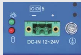
Phoenix terminal using fastening type power connector
